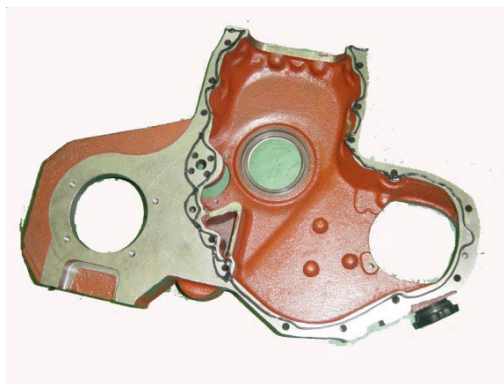
Figure 7 Sealing surface of Gear Housing
