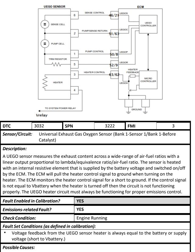
This fault will set when the UEGO heater control signal does not achieve zero volts when the heater is switched on. This may be caused by an internal fault within the ECM.
