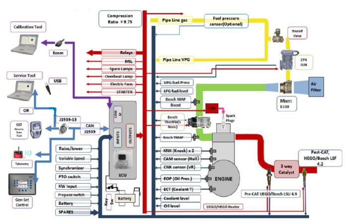
Figure 1A. 4.5L Schematic
