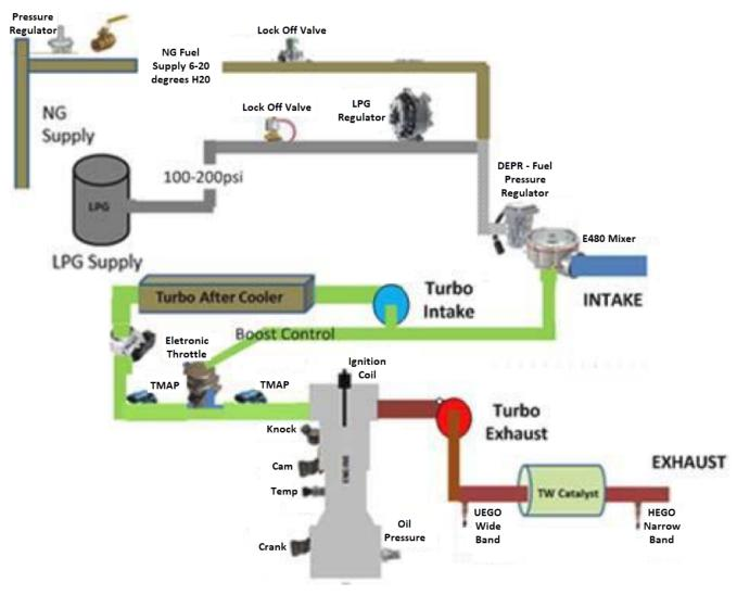
Figure 1C. 6.7L Turbo Schematic
