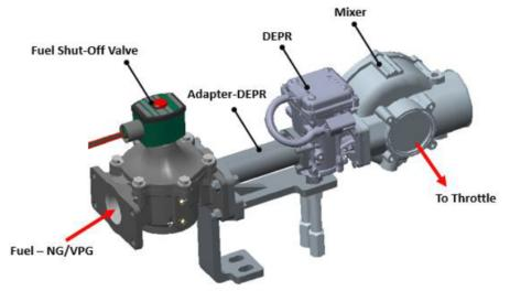
Figure 1H. 6.7L Turbo Single LPG Fuel System
