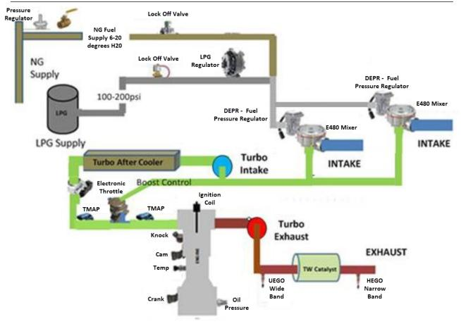
Figure 1E. 10L & 13L Turbo Schematic
