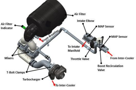
Figure 1F. 13L Turbo Air Intake System
