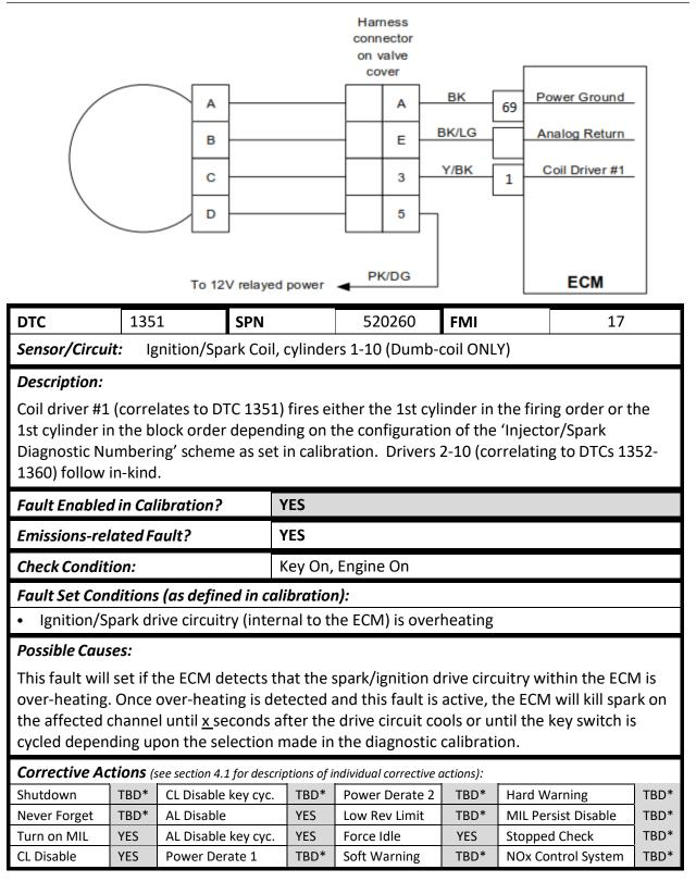
DTC 1351 – DTC 1360 – SPARK PLUG OR COIL FAILURE (CYLINDERS 1-10) (continued from previous page)
