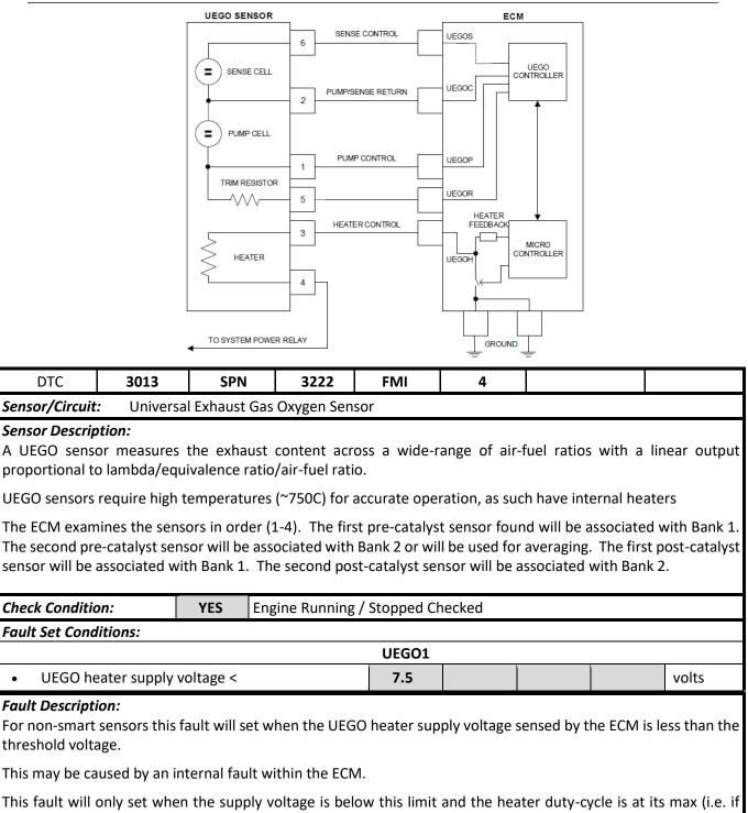
For smart sensors, the heater voltage is read by the sensor and an error communicated to the ECM if too low.
