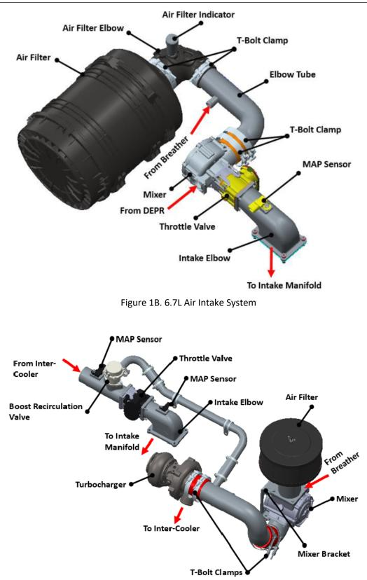
Figure 1C. 6.7L Turbo Air Intake System
