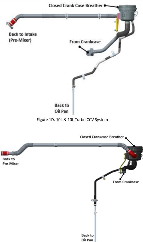
Figure 1E. 13L Turbo CCV System
