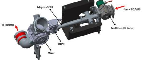
Figure 1I. 10L & 10L Turbo NG Fuel System
