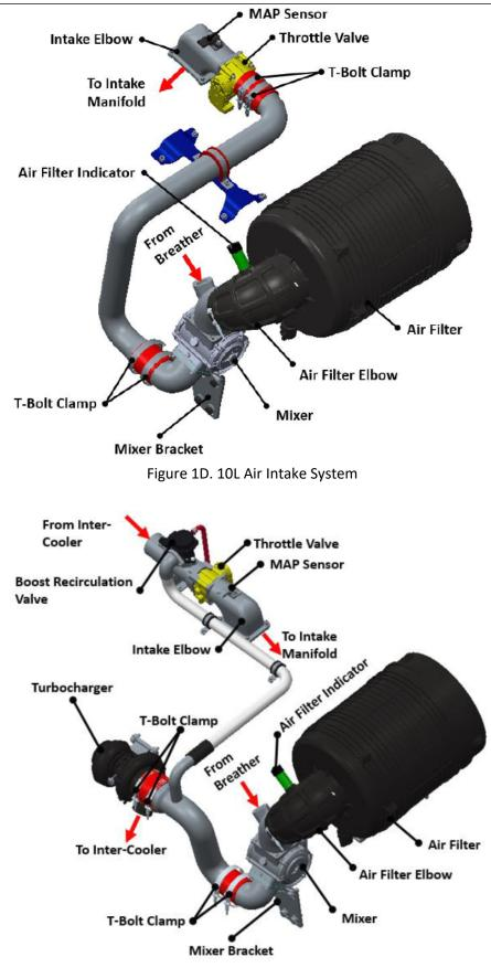
Figure 1E. 10L Turbo Air Intake System
