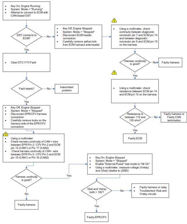
NOTE: Do not insert probe or object into terminalsas this will cause the terminal to spread and it may no longer make electrical contact with its mate. Spread pins will void warranty. Probe instead on side of terminal.
