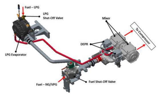
Figure 1L. 13L Turbo LPG & NG Bi-Fuel System
