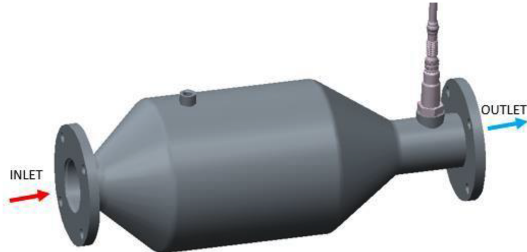
Figure 17 TWC and Post HEGO Sensor Installation
