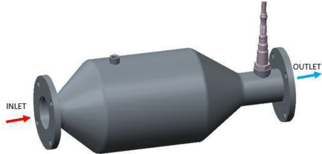
Figure 17 TWC and Post HEGO Sensor Installation
