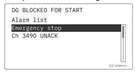
To see the other alarms, use the and buttons to go through the list. To acknowledge an alarm, select the alarm and push the button.
