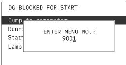
3. Use the and buttons to change the numbers, and push the button to save. Use the and buttons to move to the next number.
